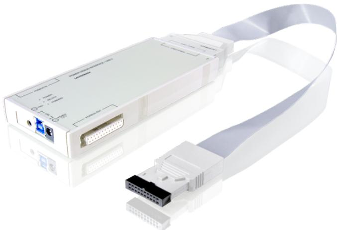
A basic debug system, generally, comprises two parts: a host connection and a target specific cable/dongle. The two pieces connect together as shown in the image to the right. The system comes with a Power Supply, USB3 cable, TRACE32 software on a DVD, and an adapter for the Trigger pin.
