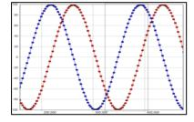
The **User Event Signal Plot** view allows you to plot any data logged as User Events. This is highly useful for analysis of control loops and other time-dependent algorithms as it allows you to correlate the data points with the other Tracealyzer views to find the cause behind anomalies in the plot. For instance, incorrect scheduling priorities or CPU overload might have delayed the computation. Double-click on a data point to find the location in the trace where the data was logged.
