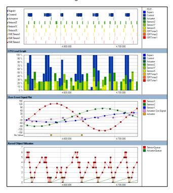
There are several supporting views with horizontal time-lines, which can be shown in a common window with synchronized scrolling. The screenshot on the left shows an example with four synchronized views:
